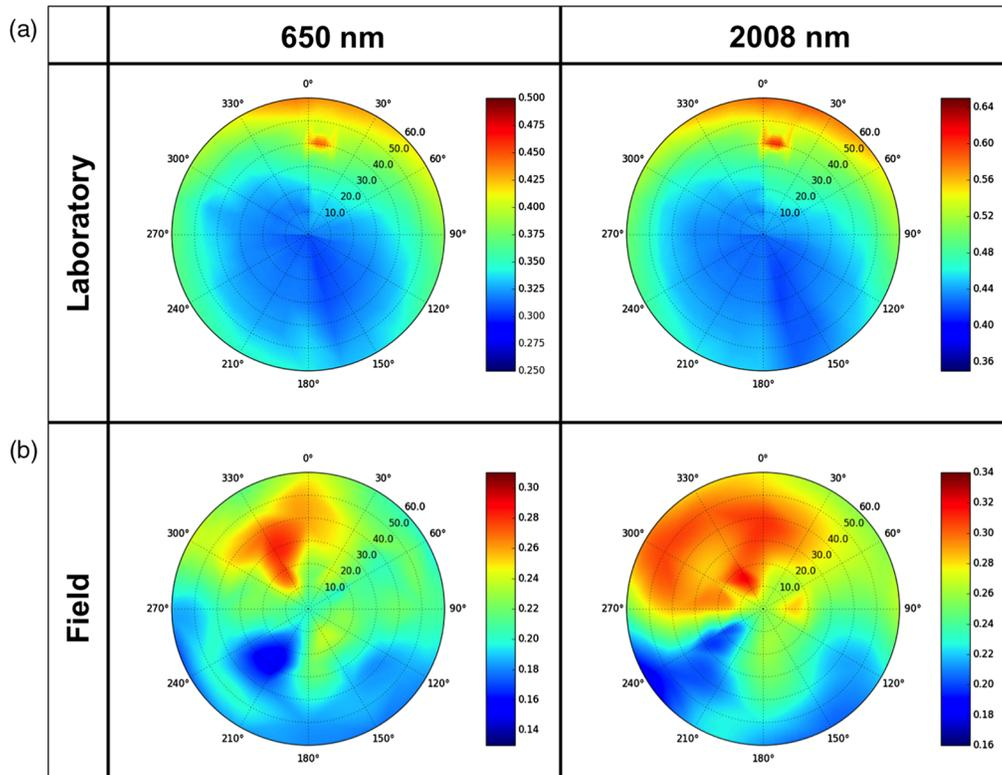
**Fig. 10** (a) BCRF data of the sediment collected from the Algodones Sand Dunes System, Brawley, California, and measured in the laboratory at RIT and (b) HCRF data of the sediment measured in the Nevada desert. BCRF and HCRF are both dimensionless quantities, which are easily seen from the definition in Eq. (1).
