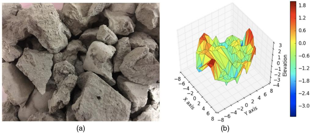
**Fig. 8** (a) Sediment collected in the Nevada desert and (b) a DEM of the sediment using the GRIT-T. The DEM has units of centimeters along the x-, y-, and z-axes. Note that the rocky appearance of the sediment surface is captured, allowing metrics of roughness to be calculated for analysis.
