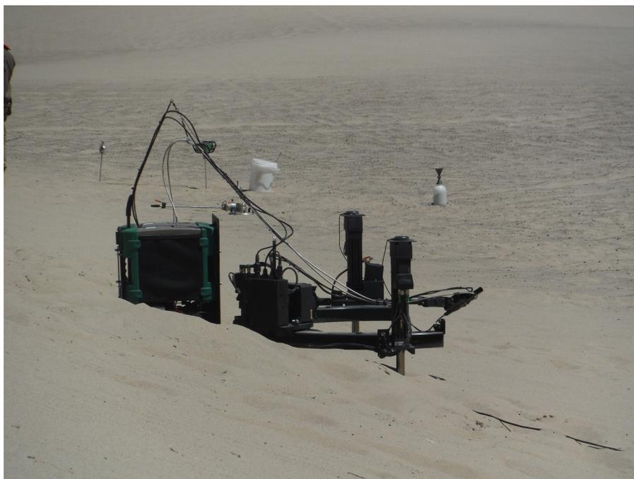
**Fig. 7** The GRIT-T as it measures the radiance reflected from a sloped sand surface. Note that the goniometric system is leveled and still able to track the same spot on the target. Also note that, on a sloped surface, the maximum zenith angle that can be reached is reduced, since the distance from the sensor to the target is enlarged.
