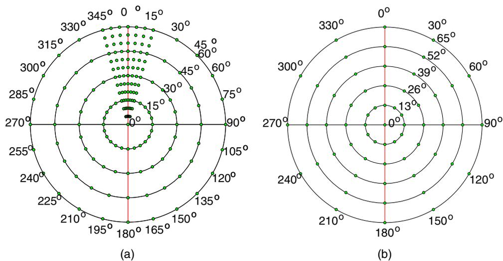
**Fig. 9** Examples of the custom-designed scan patterns for the GRIT-T in (a) a laboratory setting and (b) in a field setting. The sampled orientations are shown by the green points along the polar plot. In the laboratory example, the scan pattern has a higher measuring density around the back-scattered region of the solar principal plane, and as a result, the scan pattern has 169 view angle positions. In a field example, the scan pattern has 61 view angle positions.
