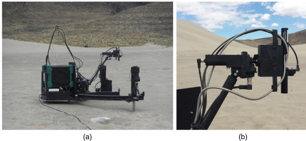
**Fig. 3** (a) Image of GRIT-T with the two ASD fiber optic cables that are guided above the shield and along the pointing arm. Once guided, the two ASD fiber optic cables are inserted into the GRIT-T pointing head, either upward or downward, and two ASD fore-optics are attached. (b) The GRIT-T pointing head with the two ASD fore-optics and ASD fiber optic cables.
