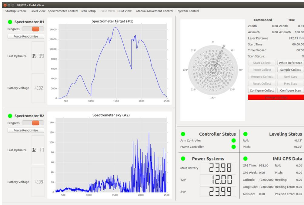
**Fig. 4** Diagnostic information during measurement observed through the GUI of the goniometer system. The interface shows the spectra in digital counts for the upward- and downward-looking spectrometers. It also monitors the progress of the generated scan pattern, the power supply, and the GPS data provided by the IMU. Shown: field view tab, one of 8 command, control, and monitoring tabs available with the GUI.
