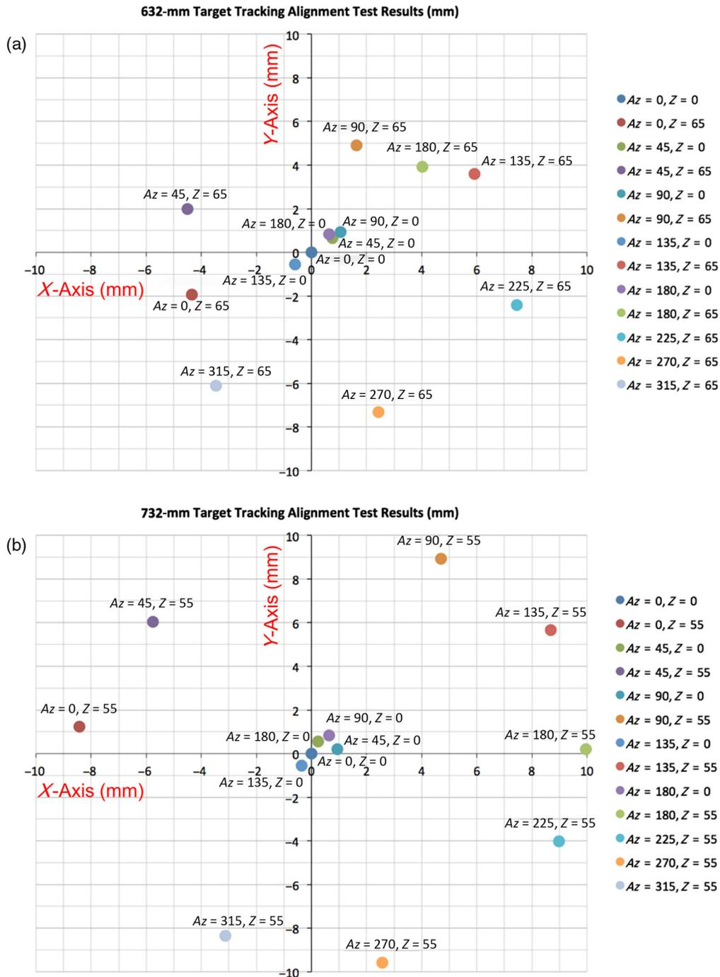
**Fig. 6** The results of performing alignment calibration operations on the GRIT-T system. These images show a coordinate system that is relative to the center of the GRIT-T C-shaped ring. Tests were done for scenarios where the sensor to target distance was (a) 632 mm and (b) 732 mm. The legend keys show the azimuth and zenith orientation of each recorded sensor orientation of the hemispherical scan pattern.
