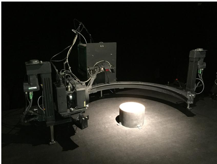
**Fig. 2** The GRIT-T instrument being operated in a dark room laboratory setting. The walls have been covered with black lab-grade felt in order to minimize diffuse scattering onto the sample of interest. In the center of the C-shaped ring of GRIT-T is a sample holder filled with sandy sediment that is being used in a laboratory study.
