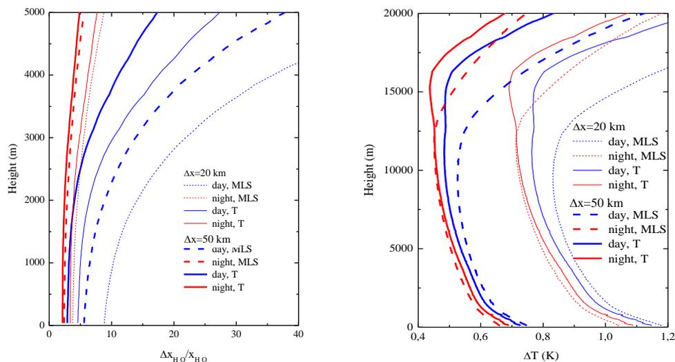
Figure 1. Vertical profiles of  $\Delta x_{H_2O}(z)/x_{H_2O}(z)$  (panel a) and  $\Delta T$  (panel b) for the tropical (continuous lines) and mid-latitude summer (dashed lines) reference models. Red lines represent night-time conditions, while blue lines represent daytime conditions. Thin lines represent a horizontal resolution of 20 km, while bold lines represent a horizontal resolution of 50 km.
