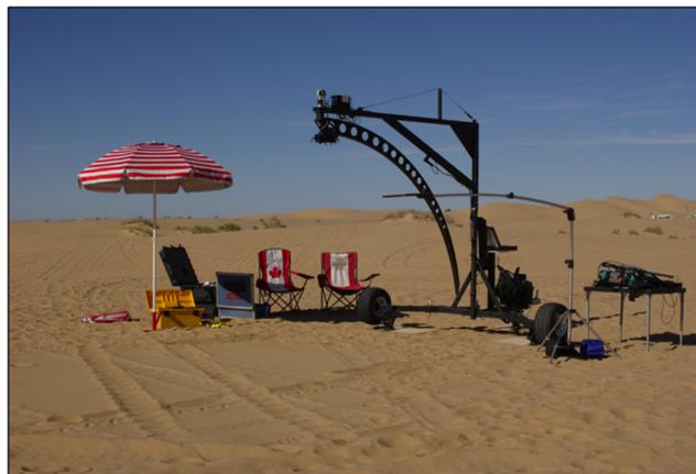
**Fig. 4** Field set-up of the ULGS II, a robotic spectro-goniometer system that has a quarter circle arc mounted to a beam that serves as a pivot for the arc, allowing for a complete hemispherical sampling of the surface from 400 to 900 nm.
