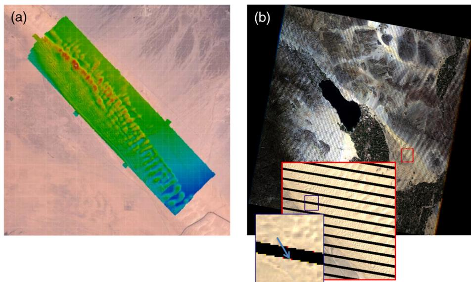
**Fig. 8** Image data collected on March 10, 2015 to support the Algodones Dunes system campaign. (a) The LiDAR data collected with G-LiHT. (b) An RGB image of the Landsat 7 data collected with ETM+. Note that the BRDF ground locations shown in the zoom window in Fig. 7 fell at the edge and within the scan line gap of the image data as indicated with the arrow.
