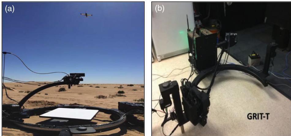
**Fig. 3** (a) The first generation GRIT that was deployed during the Algodones Dunes system campaign. (b) The second generation GRIT-T that was developed after the campaign and used to process core samples.
