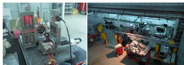
Fig. 2. CCD272-64 EQM Enclosure at "Kosmos" metrological station (VEPP-4M synchrotron) during quantum efficiency measurements (INP, Novosibirsk, Russia).
