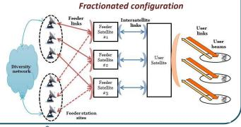
The fractionation concept brings a new VHTS product **MATRIX** to life for the next decade. It reduces the cost and complexity of the feeder segment and offers the possibilities of progressive deployment and risk-free upgrade from a radio transparent VHTS to an optical regenerative VHTS.
