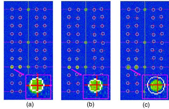
Fig. 2 Fine-tuning for probe classification. Red crosses are the initial spot positions predetermined by the located marker. White circles denote the final spot areas. (a) No search, the white circle is centered at the cross point; (b) position search, the white circle is not centered at the cross point; and (c) position and size search, the white circle is not centered at the cross point and its size is greater than the initial size.
