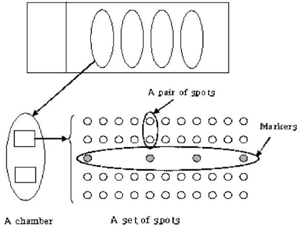
Fig. 1 Architecture of HPV DNA chip microarray.
