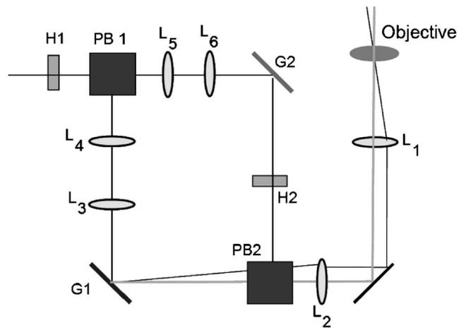
Fig. 1 Double optical tweezers system.
