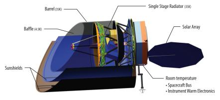
**Fig. 3** Origins temperature zones are designed to maximize cryo-cooling efficiency while ensuring a 4.5 K environment for the telescope and instruments. The instruments are housed in the 4.5 K zone beneath the primary mirror. The 35 K radiator is more clearly shown in Fig. 5.
