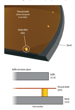
Fig. 6 Schematic of mounts of 20 K shield to the inside of the 35 K barrel.
