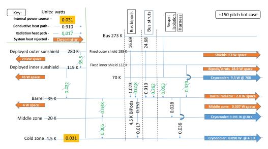
**Fig. 8** Origins heat flow map shows that multiple stages of cooling results in a reasonably small heat load to the cryocooler and radiative cooler stages.
