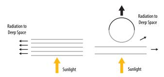
Fig. 2 A two-layer sunshield plus radiator can achieve the same radiative temperature as a five-layer sunshield.
