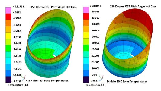
**Fig. 10** The 4.5 K shell and 20 K shield temperature contours remain nearly isothermal even for the worst case, 150-degree pitch attitude.
