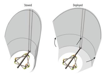
**Fig. 7** The two-layer sunshield is deployed by releasing the layers from the barrel and pushing them outward from the base. Only the outer layer is shown for clarity.
