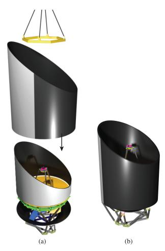
**Fig. 5** (a) The Origins barrel is shown being lowered over the telescope and baffle assembly. (b) The assembly comprises the CPM, which can be structurally and thermally tested as a unit.
