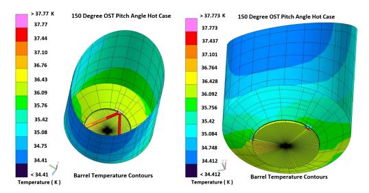
**Fig. 11** The barrel temperature contours show that the barrel temperature remains below 36 K and nearly isothermal in the worst-case attitude (150° pitch) over nearly all of its surface.
