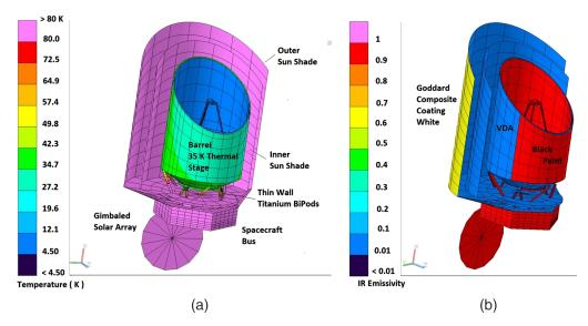
**Fig. 9** (a) A Spitzer-like architecture with staged cooling, a two-layer sunshield, a deep space radiator, and cryocoolers delivers the required thermal performance with a relatively simple-to-model design. (b) The temperature map and right shows the emissivities used to create the model.
