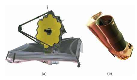
Fig. 1 The Origins architecture is more like (b) Spitzer than (a) JWST.
