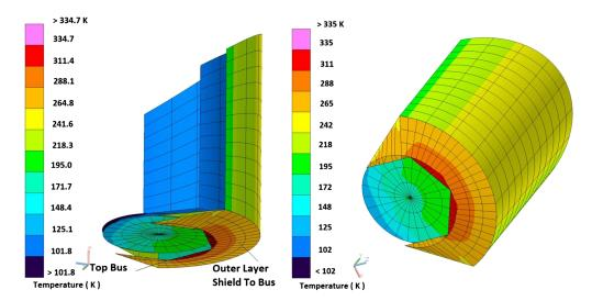
Fig. 12 The outer sunshield with GCC maintains room temperature or lower for all FOR over nearly all of its surface.
