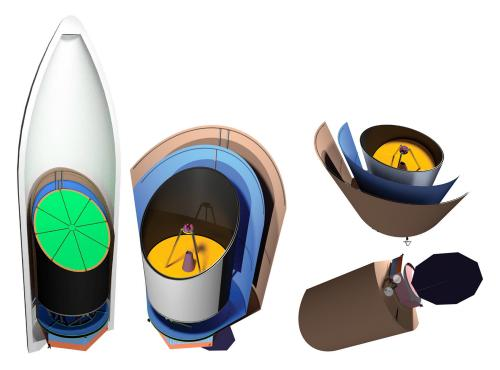
**Fig. 4** The left side depicts Origins in the stowed configuration in the SLS fairing with sunshields wrapped around the barrel and ejectable cover, and the right side shows three different views of the fully deployed observatory.
