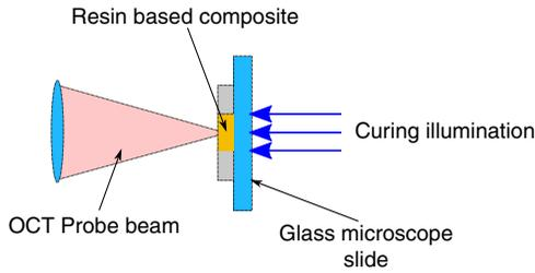
**Fig. 1** Experimental configuration. The resin-based composite was constrained within a 0.75 mm deep, 4 mm diameter ring placed on a glass microscope slide through which the OCT probe beam and the curing lamp illuminated the sample.
