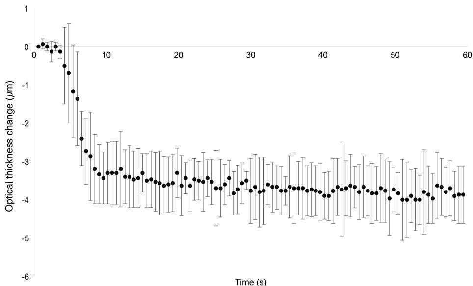
**Fig. 2** Mean optical thickness change for the three dental composite specimens measured over a 60 s period. Error bars represent 95% CIs for the mean thickness change over three independent experiments.
