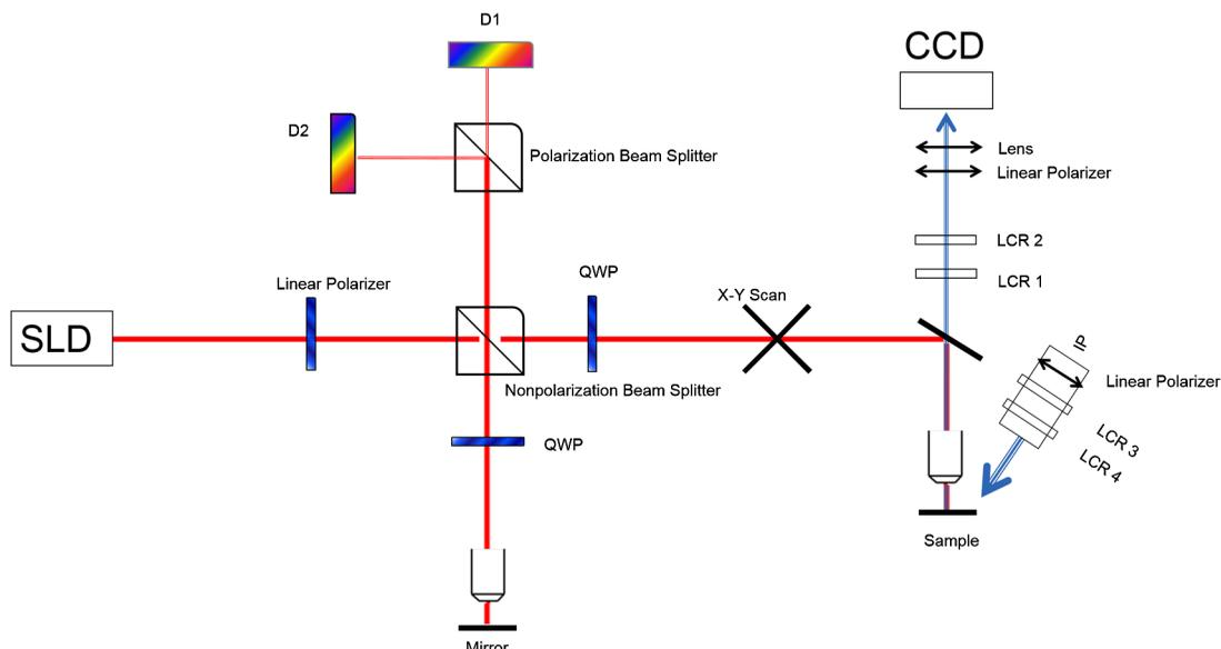
Fig. 1 Combined PS-OCT and Mueller matrix polarimeter schematic.
