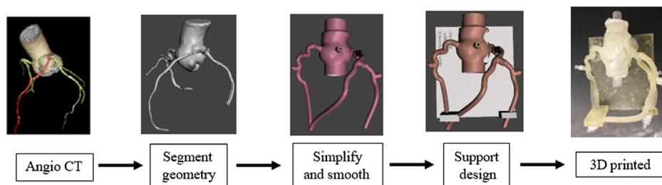
**Fig. 1** Five key steps in phantom design process, starting with CT angiography images from the patient, segmentation of the desired geometry, simplifying and smoothing of vasculature, designing a support for the vasculature and appending it, then finally 3D printing the phantom.
