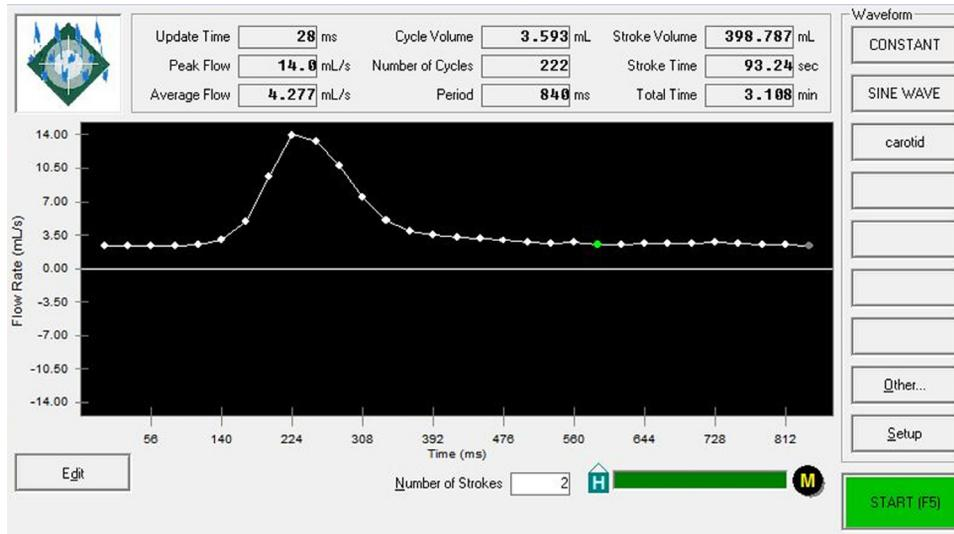
Fig. 2 Waveform used with the CompuFlow 1000 programmable pulsatile pump.
