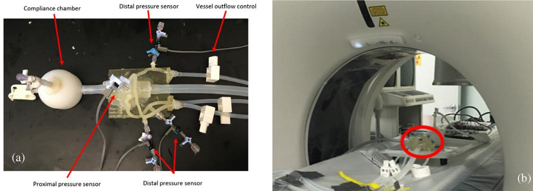
**Fig. 4** Benchtop setup of 3D printed patient-specific phantoms. (a) Phantoms in established flow loop with programmable pulsatile pump with pressure sensors attached and (b) phantom, outlined in red, in Aquilion ONE scanner for CCTA scans.
