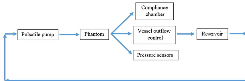
Fig. 3 Overview of key components of flow loop for experimentation. Blue arrows represent the direction of flow.
