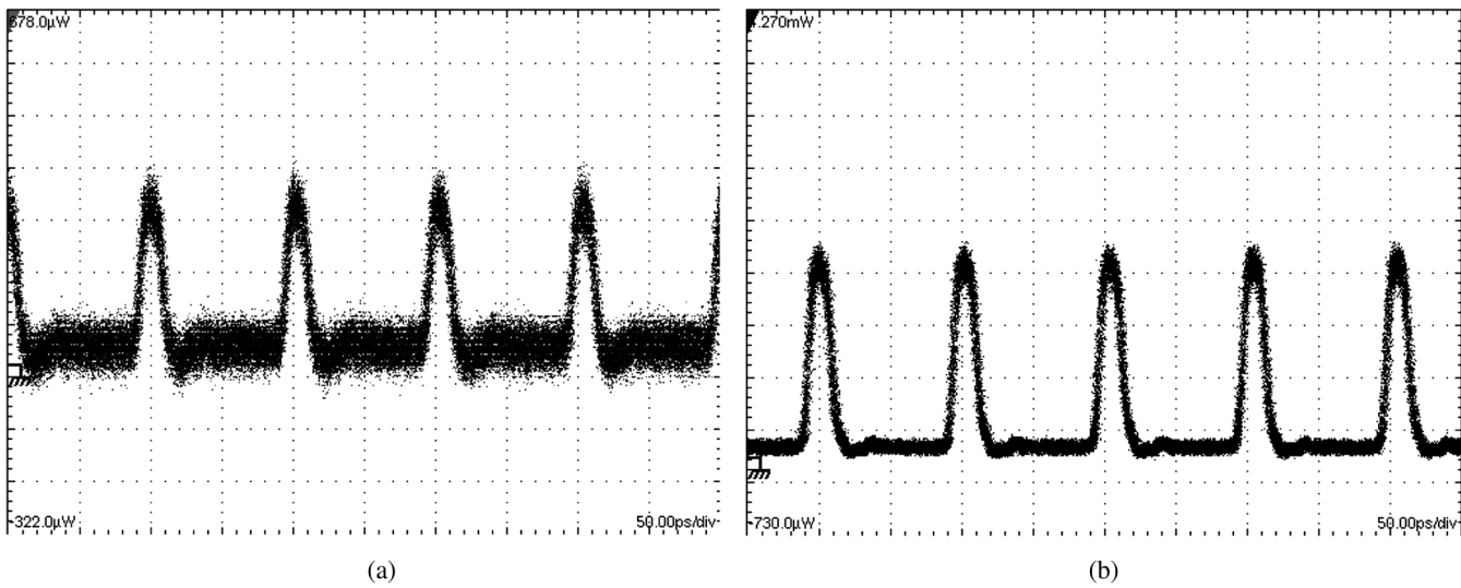
Fig. 3 Pulse profiles of (a) pump, and (b) probe after wavelength conversion.
