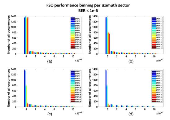
**Fig. 10** Azimuthal variations in 2016 FSO performance binning of BER of  $1 \times 10^{-6}$  or less for (a) 20-deg, (b) 40-deg, (c) 60-deg, and (d) 80-deg zenith angles.
