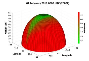
**Fig. 5** February 1, 2016, 0000 UTC weather cube displaying BER by azimuth and zenith angles. Note that high BERs (red) across the dome are due to cloud cover.
