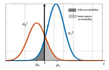
Fig. 3 Receiver output distribution under Gaussian noise assumptions.
