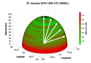
**Fig. 4** Weather cube, centered on the NCR, displaying BER by azimuth and zenith angles on January 7, 2016, at 1200 UTC. The color scale indicates high (red) and low (green) BERs. The white arrows correspond to the five zenith angles evaluated for 2016 FSO performance binning.
