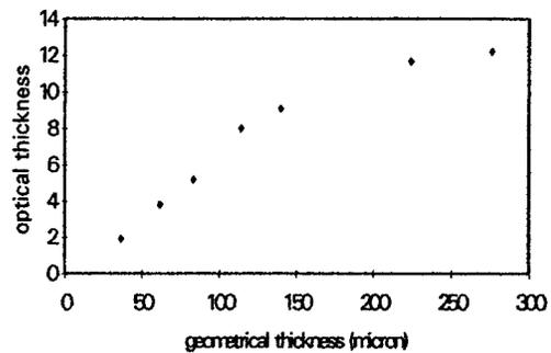
**Fig. 1** Limits due to multiple scattering on the determination of the extinction coefficient. The curve refers to attenuation measurements carried out on a highly packed diffusing medium (water and polystyrene spheres  $\Phi = 1.5.8 \mu\text{m}$ , concentration 20%). In this case the optical depth versus the geometrical thickness is a straight line, with the angular coefficient equal to  $\mu_e$ , for  $\tau_m$  smaller than about 11.
