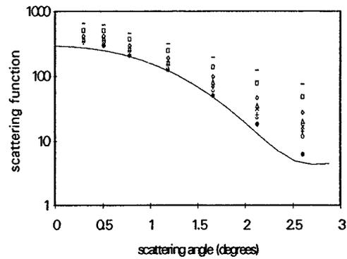
**Fig. 4** Effect of multiple scattering on measured scattering functions for polystyrene spheres with  $\Phi=11.9 \mu\text{m}$ . Symbols refer to different optical depths: from lower to upper:  $\tau_m=0.38, 1, 1.3, 1.6, 1.9, 2.6, 3.7,$  and  $4.7$ , respectively. The solid line is calculated from Mie theory.
