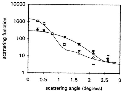
**Fig. 3** Tests of the measuring method for  $p(\vartheta)$ . The figure shows a comparison between experimental results obtained from measurements carried out on polystyrene spheres and the results of Mie theory (continuous lines). Two different sizes have been used:  $\Phi=11.9 \mu\text{m}$  (solid symbols) and  $\Phi=25 \mu\text{m}$  (hollow symbols). The optical depths were 0.38 and 0.7, respectively.
