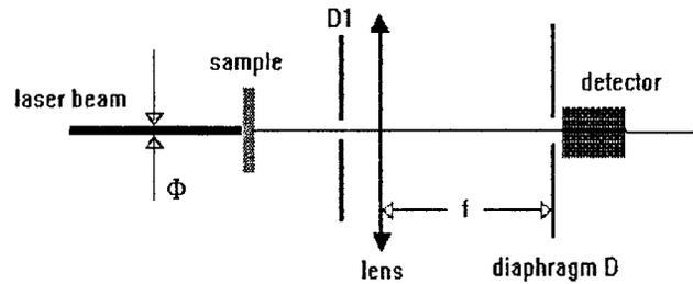
**Fig. 2** Scheme of the experimental setup. The light beam was an He-Ne laser. The diaphragm D with radius R was placed in the focal plane of the lens in front of the detector.
