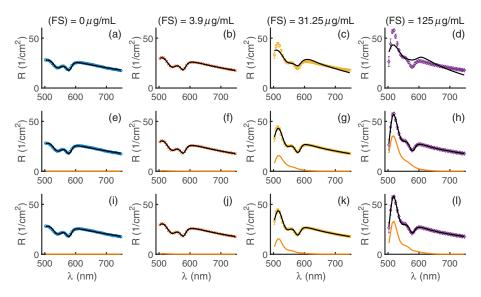
**Fig. 2** Reflectance spectra and model fits with constant background optical properties (BVF = 2%, LVF = 1.5%) and variations in FS. Data show differences in fit quality for (a)–(d)  $R^M$ , (e)–(h)  $R^M_E$ , and (i)–(l)  $R^M_{AE}$ . Black lines are model fits to data, and orange curves are the components of reflectance due to FS emission for  $R^M_E$  and  $R^M_{AE}$ .
