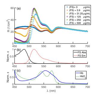
Fig. 1 (a) Reflectance spectra data sampled in optical phantoms with constant background optical properties (BVF = 2%, LVF = 1.5%) over a range of FS concentrations with variations in spectra dependent on emissions of FS. (b) The absorption and emission spectra for fluorescein and (c) absorption spectra for oxy- and deoxyhemoglobin incorporated into the fitting are shown, normalized to their respective peaks.
