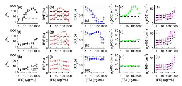
**Fig. 3** Reduced chi-squared and optical parameter estimates from (a)–(e)  $R^M$ , (f)–(j)  $R^M_E$ , and (k)–(o)  $R^M_{AE}$  from measurements of optical phantoms with constant scattering (1.5% LVF), and variation in both BVF = (1,2,3)% and FS (0.98 to 1000  $\mu$ g/mL). For  $\chi^2/\nu$ , the dashed line represents the zero-FS case. For all other plots, the dashed line represents known value.
