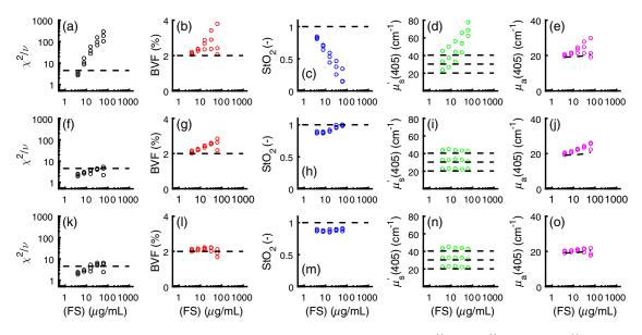
**Fig. 4** Reduced chi-squared and optical property estimates from (a)–(e)  $R^M$ , (f)–(j)  $R^M_E$ , and (k)–(o)  $R^M_{AE}$  for phantom data exploring changes in scattering, with LVF = (11.52)%, BVF = 2%, and FS (3.9 to 62.5  $\mu$ g/mL). For  $\chi^2/\nu$ , the dashed line represent the zero-FS case. For all other plots, dashed lines represent known values.
