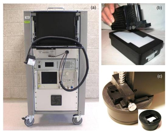
Fig. 1 (a) DOSI instrument and (b) and (c) illustrate the probe placed on the calibration phantom (FDPM calibration) and on the reflectance standard (broadband calibration), respectively.
