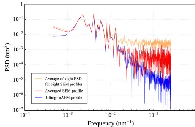
**Fig. 6** Average of eight PSDs for eight SEM profiles (orange), PSD of the averaged SEM profile (red), and PSD of the tilting-mAFM profile (blue).
