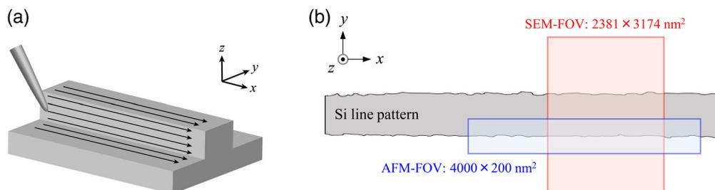
**Fig. 1** (a) Illustration of the fast scan direction along the line pattern. The 3D sidewall shape is scanned from the bottom to top surface through the sidewall by the tilting-mAFM. (b) The FOVs of the SEM and tilting-mAFM overlapped for the direct comparison.
