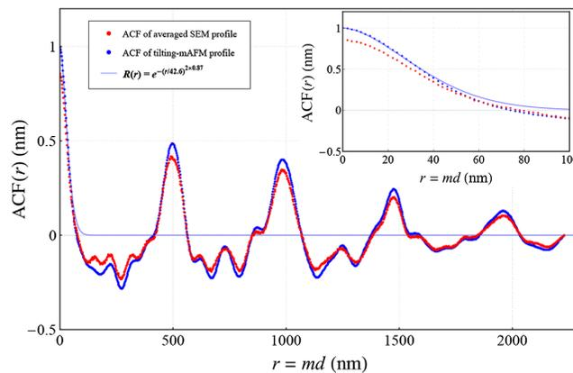
**Fig. 8** Plot of the calculated ACFs for the averaged SEM profile (red dots) and the tilting-mAFM profile (blue dots), and the model autocorrelation function for the tilting-mAFM profile (light blue line). The inset is an enlarged plot of part of the x axis.
