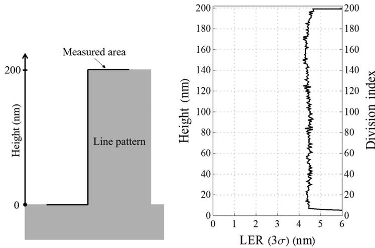
**Fig. 5** LER ( $3\sigma$ ) distribution along height.
