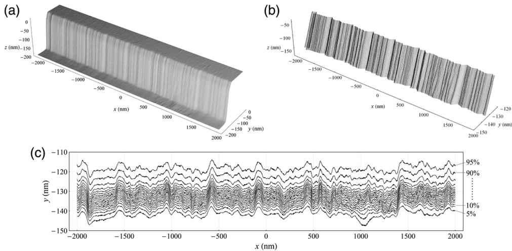
**Fig. 3** (a) AFM image of a sidewall expressed as a 3D point cloud. The scale of each axis is modified for visibility. (b) An enlarged sidewall image of (a). (c) Line-edge profiles ( $xy$  plot) at every 5% height ( $z$ ) interval from 5% to 95%.
