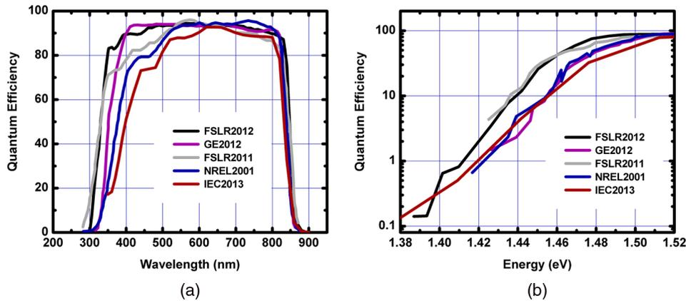
**Fig. 2** (a) Quantum efficiency (QE) versus wavelength comparison of five different cells. (b)  $\log_{10}$  QE versus energy data for the cells of (a).
