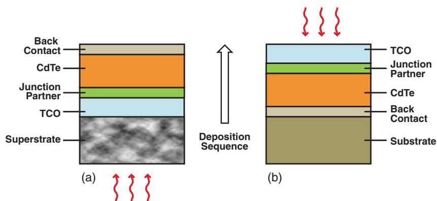
**Fig. 1** CdTe solar cell configurations: (a) superstrate and (b) substrate.
