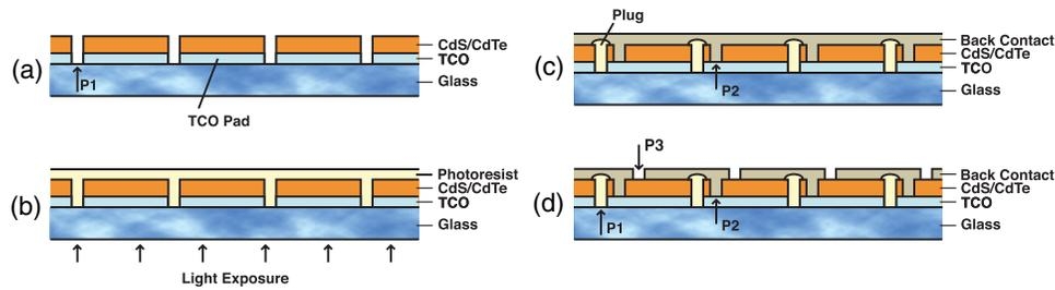
**Fig. 4** Photoresist plug integration process flow for monolithic integration: (a) deposit TCO/CdS/CdTe stack and form P1 scribe lines, (b) cover the surface with photoresist and expose through the glass superstrate, (c) develop and rinse forming the photoresist plugs, form P2 scribe lines, deposit back contact, (d) form P3 scribe lines.
