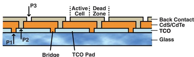
**Fig. 3** Module structure with a CdTe bridge between transparent-conductive-oxide (TCO) pads.
