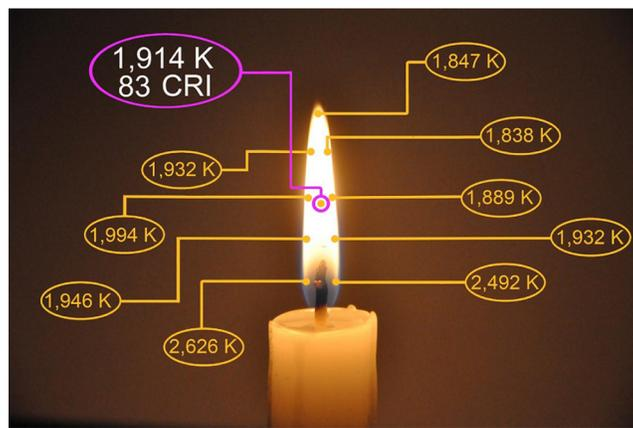
**Fig. 1** Candle shows different color temperatures (CTs) at different positions inside the flame. The CT varies from 1847 to 2626 K for the white candle studied herein. To represent, the CT of the brightest spot is chosen, which is 1914 K (Ref. 18).
