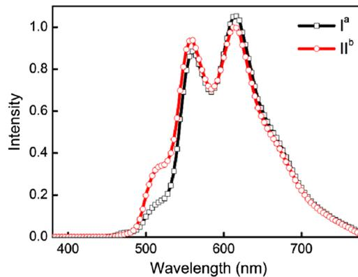
**Fig. 4** Electroluminescent spectra of no and neat CML-composing counterparts. (a) With no CML, (b) a 2-nm neat TCTA as interlayer. All spectra were obtained at 5 A/m<sup>2</sup>.
