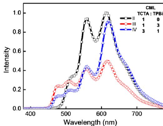
**Fig. 5** Electroluminescent spectra of the blend CML-composing devices.
