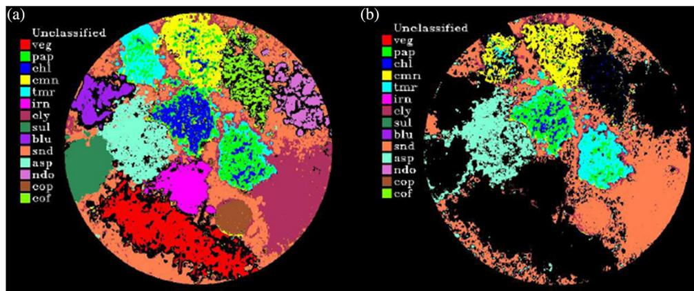
**Fig. 6** The classified microscenes are shown with false colors representing each class. (a) The original microscene and (b) the wavelength error classified microscene.
