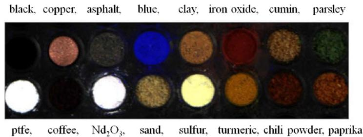
**Fig. 4** A normal color composite using spectral bands 641, 549, and 458 nm for red, green, and blue, of the 96-well sample tray (microarray) filled with the materials used in the microscene. The black is an empty cell in the sample tray.
