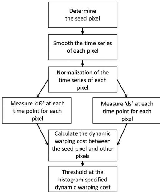
Fig. 4 Block diagram of the similarity algorithm.
