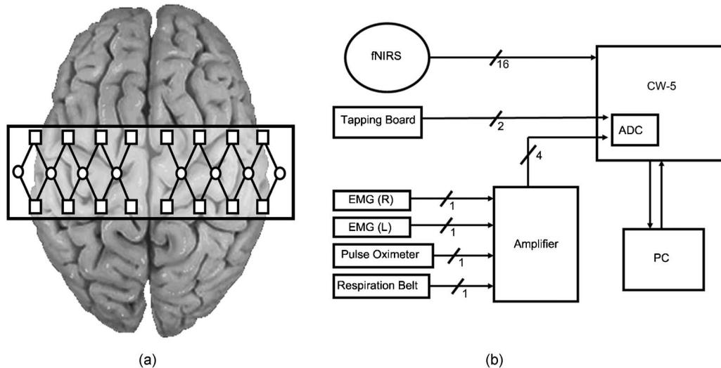
**Fig. 1** (a) Placement geometry of the fNIRS probes over the motor cortex. The circles represent sources, and the squares represent detectors. (b) Overall instrumentation setup.
