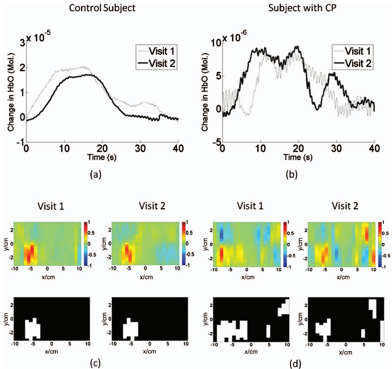
**Fig. 11** Repeated fNIRS measurements for a control (Subject 2) and a subject with CP (Subject 8) performing right finger tapping: (a,b) show the time-series reflectance patterns for the same source-detector pair, while (c,d) show the activation images (top) and their corresponding activation-threshold images (bottom) for each visit.
