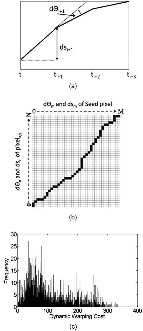
**Fig. 3** (a) Measurements made for the change in angle defined by the tangent ( $d\Theta$ ) and the change in amplitude ( $ds$ ) for every time point, (b) illustration of a DTW path, and (c) histogram of the dynamic warping costs for all control subjects.
