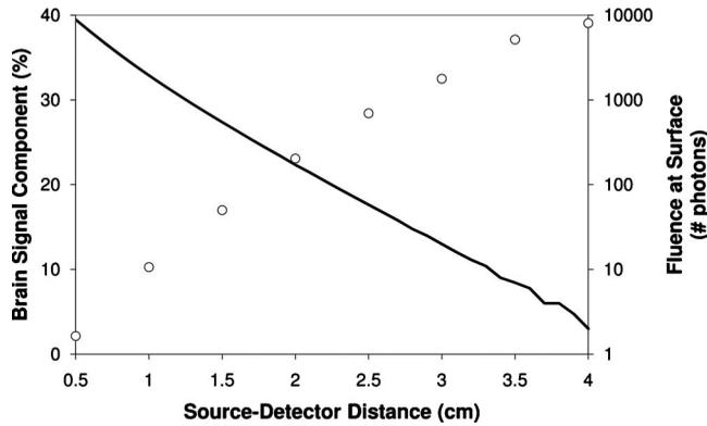
**Fig. 1** Relative brain signal component (open circles) as a function of source-detector distance for Monte Carlo simulations performed using the optical properties in Table 1 and assuming an ECL thickness of 10 mm. The corresponding fluence at the surface of the head for  $10^8$  simulated photons is shown on the right axis (solid line), illustrating the tradeoff between penetration depth and signal intensity.
