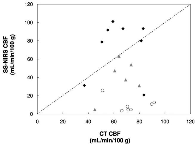
**Fig. 5** Correlation plot comparing the CT and SS-NIRS measurements of CBF. Symbols represent three ECL groups described in Fig. 4. No significant correlation between the two measurements was detected. The dashed line indicates the line of unity.
