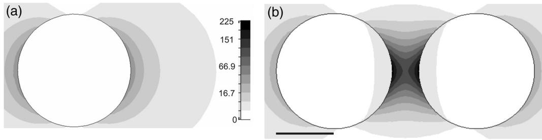
**Fig. 1** Numerical simulation of electric field intensity ( $E^2$ ) for a monomer (a) and dimer (b) for 100 nm diameter gold NPs and an interparticle spacing of 23 nm. The incoming light was horizontally polarized at a wavelength of 640 nm. Scale bar is 50 nm.
