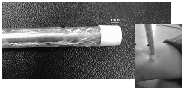
Fig. 1 Image showing the reflectance fiber optic probe used indicating the separation distance introduced and as applied on a participant.
