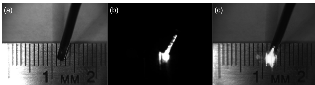
Fig. 7 NIR laser light delivered through handheld laser wand for demonstration of NIR laser beam guidance by augmented microscope: (a) visible image conceals location of NIR laser beam, (b) NIR image lacks any spatial information, and (c) augmented image visualizes both NIR light and visible spatial cues.
