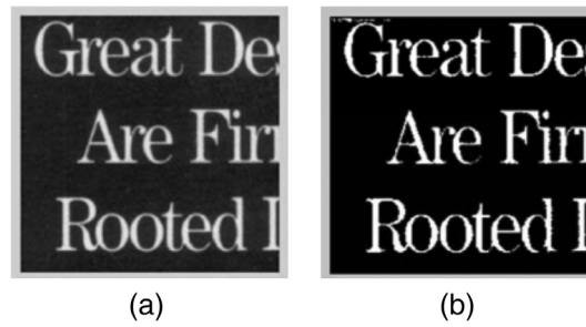
Fig. 6 Image thresholding using Bernsen's local thresholding method: (a) original image and (b) image after thresholding with l = 15 and w = 3 . 35
