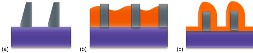
**Fig. 1** Process-embedded asymmetry. (a) Asymmetric sidewall angle caused by etch. (b) Asymmetric trench caused by chemical-mechanical polish (CMP). (c) Asymmetric layer deposition caused by chemical vapor deposition (CVD) deposition.
