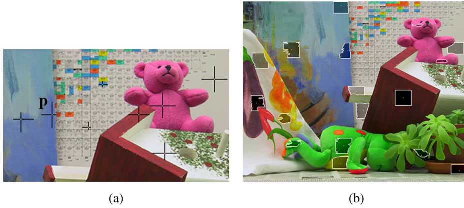
Fig. 2 Construction of cross skeleton and local support region on Teddy image: (a) pixel-wise adaptive cross skeleton at pixel \mathbf{p} and (b) sample shape-adaptive support regions.
