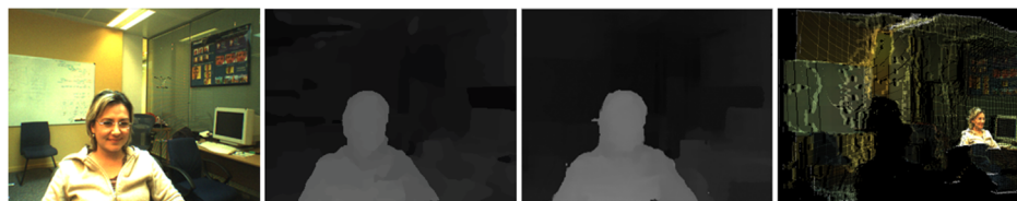
Fig. 10 Snapshots of Ilkay stereo sequence from Microsoft i2i database: (a) reference frame. Disparity result by (b) aggregation with enhanced segment tree 30 (c) proposed method; and (d) 3-D reconstruction view of (c).
