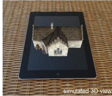
Figure 6: The phantoView system – 3D object models loaded into the system are rendered in real-time as phantograms to the tablet's display. A rendered object appears to be sitting on the tablet's surface. Rotating the tablet about the vertical axis allows the object to be seen from other viewpoints.
