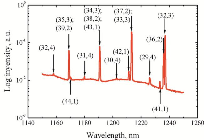
Figure 6. Low-temperature luminescence spectrum of the microring. Estimated mode orders  $\text{TE}_{m,n}$  are indicated near the peaks.
