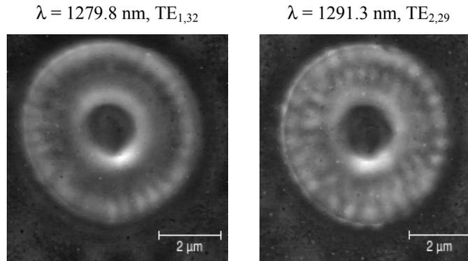
Figure 7. NSOM images demonstrating WGM modes of different orders in the microring resonator.
