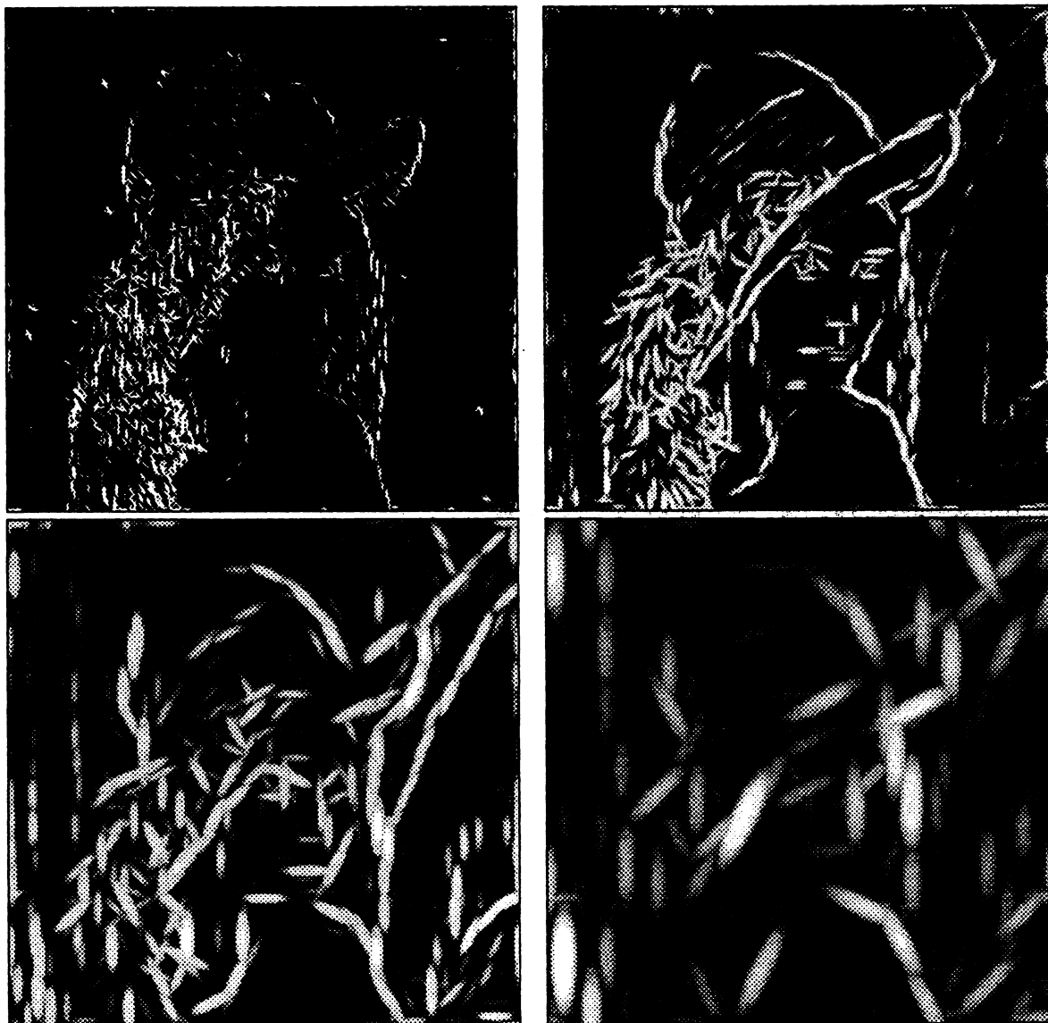
Figure 2: Symbolic representation of the Gabor vectors: each atom is symbolized by an elongated Gaussian of width proportional to the scale 2^j , oriented along the modulation direction, of gray level proportional to its amplitude. Light atoms correspond to high amplitude. The images from left to right and from the top to the bottom corresponds to the scale 2^1 to 2^4 .
