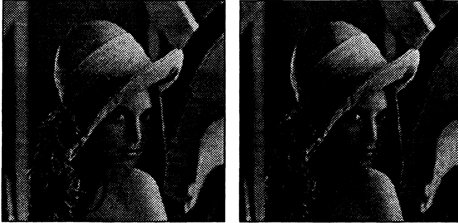
Figure 3: Original Lena image (left figure) and reconstruction with 2500 (right figure). The reconstruction is obtained as a truncated sum of the decomposition.
