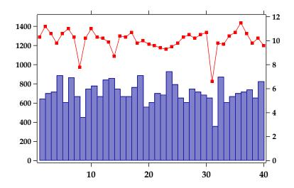
Figure 3. Reproducibility of the pump laser energy for the second target (vertical bars) and the x-ray laser energy (red closed circles). The vertical scale on the right-hand side shows the pump laser energy in J, and the vertical scale on the left-hand side shows the x-ray laser energy in nJ normalized by the divergence in mrad<sup>2</sup>. The horizontal axis is the consecutive shot number.
