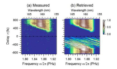
Figure 6. Time-resolved reflection spectra of the vuv pulse. (a) shows the measured PM-FROG trace, whereas (b) shows the retrieved FROG trace after iterative calculation with PCGPA. The noise at  $\tau < 0$  in (b) is an artifact since only  $\tau \ge 0$  has been retrieved in this calculation.
