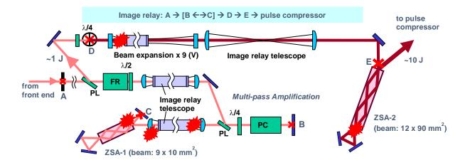
Figure 2. Optical layout of one beam of the zig-zag slab laser system TOPAZ for x-ray laser pumping. The rectangular beam pattern at the soft aperture at A is relayed to B, C, D and E by the image relay telescopes. The locations susceptible to laser damage are marked by stars. Acronyms are PL: polarizer,  $\lambda/2$ : half-wave waveplate,  $\lambda/4$ : quarter-wave waveplate, FR: Faraday rotator, and PC: Pockels cell.
