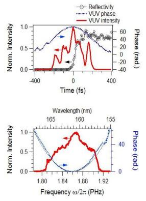
Figure 7. Upper figure shows the time-resolved intensity (solid curve) and phase (dotted curve) of the vuv pulse and the time-resolved reflectivity of the plasma mirror (open circles), both determined by PM-FROG. Lower figure shows the frequency dependence of the intensity (solid curve) and phase (dotted curve) of the vuv pulse, where the thin solid curve shows the calculated phase change of the vuv pulse due to propagation in a LiF lens of 2.3 mm thickness.
