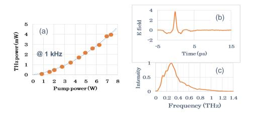
Figure 5. Properties of THz radiation generated with QUADRA-T laser: (a) THz power vs pump laser power, (b) time dependence of the electric field of THz radiation, and (c) spectral intensity of THz radiation. (Vertical axes in (b) and (c) are in arbitrary scales.)
