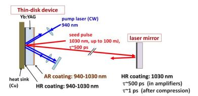
Figure 4. Layout of a Yb:YAG ceramic thin-disk amplifier pumped by cw LD at 940 nm. The thin disk has 200-µm thickness and 10-mm diameter, in which central area of 6-mm diameter is doped with Yb.
