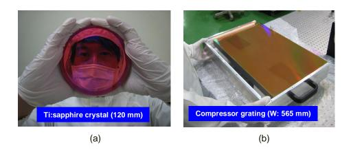
Figure 1. Photographs of (a) a 120-mm diameter Ti:sapphire crystal and (b) a gold-coated diffraction grating with 565-mm width used for upgrading J-KAREN laser.
