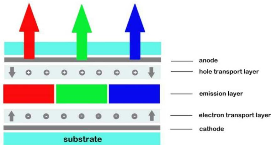
Figure 2. Schematic diagram of the OLED technology [16]-[19]
