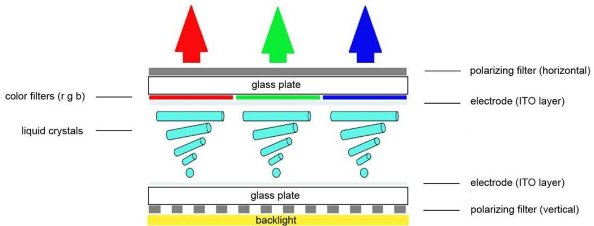
Figure 1. Schematic diagram of the LCD technology [4]-[6]
