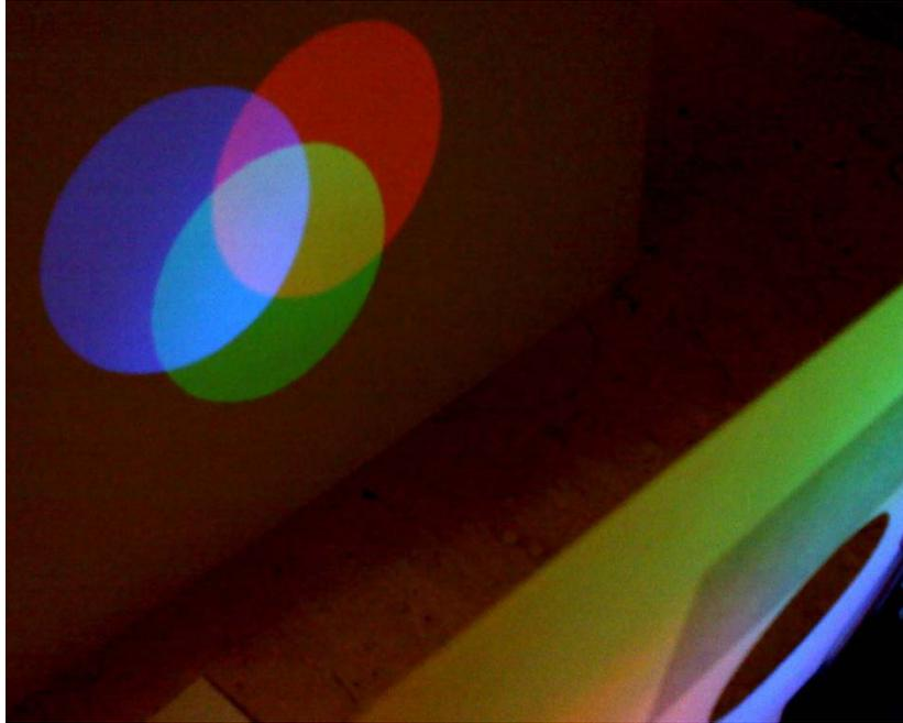
Figure 3. RGB color mixing triangle. These are produced by placing the three colored LED's close together and then having their light pass through a circular aperture.
