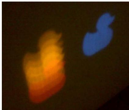
Figure 7. Comparison image of light through a duck shaped aperture. On the left, we see the image from the array of LED's. On the right, we see the image from a single blue LED. In the array, the red LED is at the top of the array.
