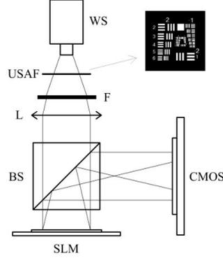
Fig. 1. Scheme of the FINCH experimental system. WS, white light lamp; USAF, object; F, interference filter; L, lens; BS, beam splitter; SLM, spatial light modulator; CMOS, digital camera.
