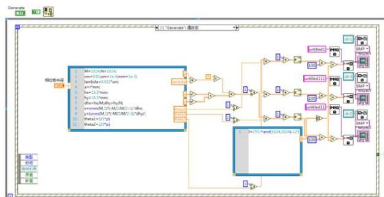
Fig. 2. Original graphical program code for DOE generation.
