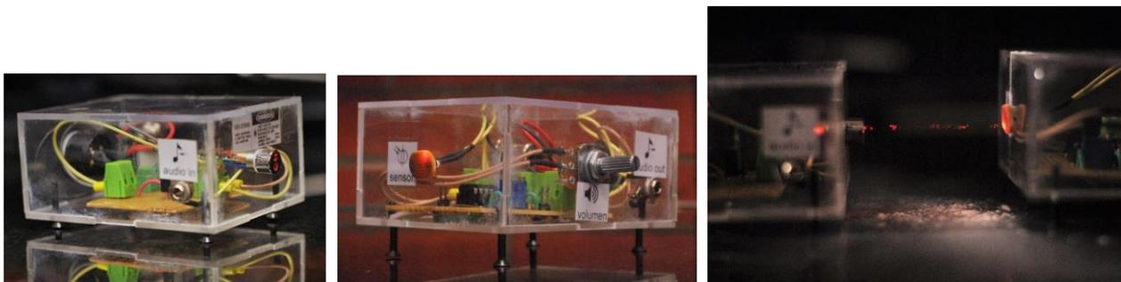
Figure 6. Pictures of our *optophonograph*. From left to right: a) transmitter, b) receiver, and c) transmitter sending signal to receiver. Signal enters the transmitter through an audio jack from any music player device, and alters the intensity of the laser. The receiver reads the laser signal with a photoreistor, and sends the electrical signal to an external speaker or earphones through an audio jack. Volume can be set in the receiver.
