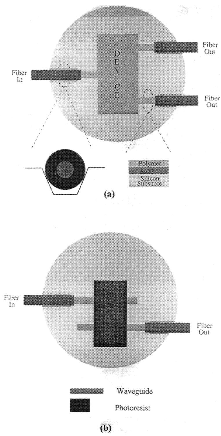
Fig. 4 Schematic diagram of (a) substrate with V-grooves for fiber optic coupling and (b) photoresist directional coupler.
