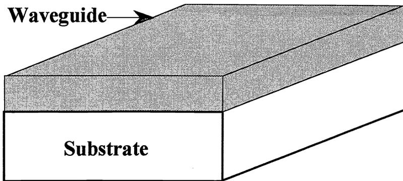
Fig. 2 Optical waveguide formed by spinning photoresist on glass substrate.
