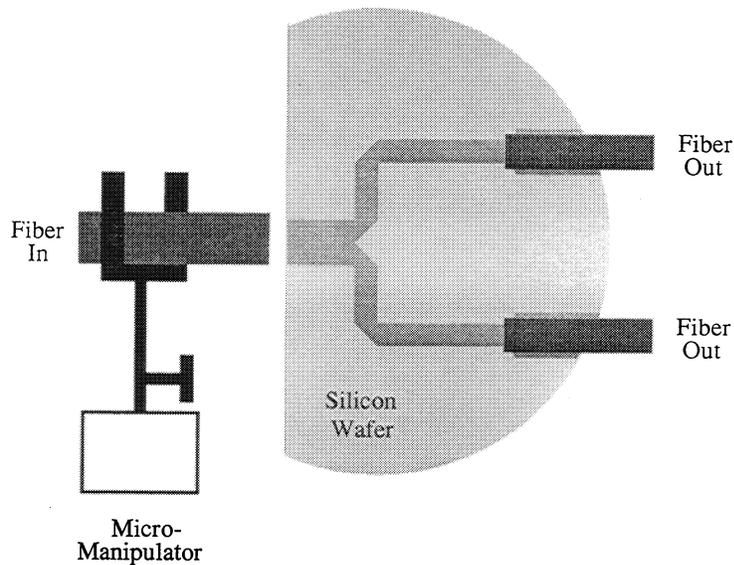
Fig. 6 Fiber end fire coupling to the optical power divider.
