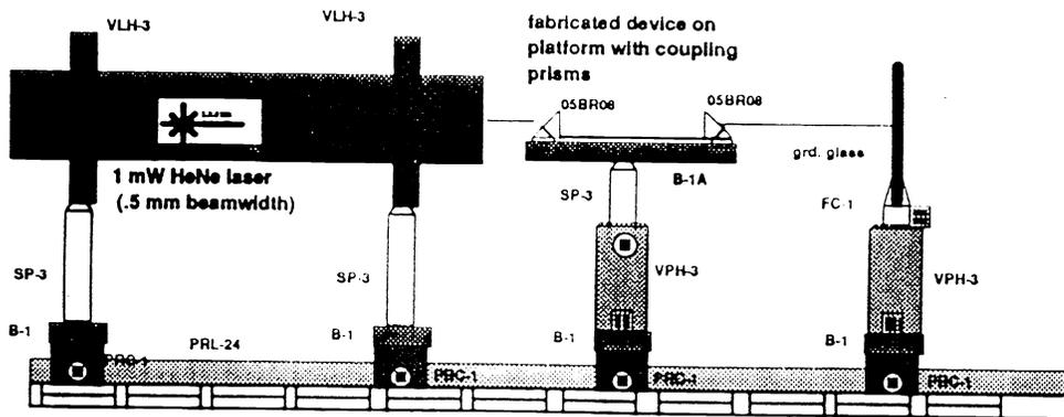
Fig. 3 Experimental setup for waveguide characterization.
