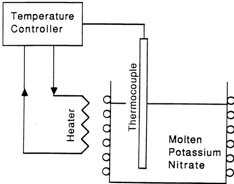
Fig. 1 Schematic diagram of the ion-exchange apparatus.
