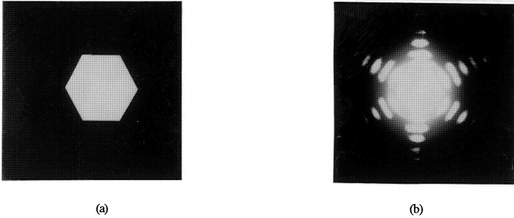
Fig. 5. Hexagonal diffracting object (a) and its Fraunhofer diffraction pattern (b).
