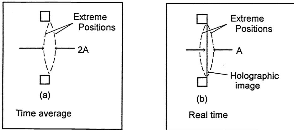
Figure 3. Recorded Diaphragm Displacement a) Time Average Holography b) Real Time Holography
