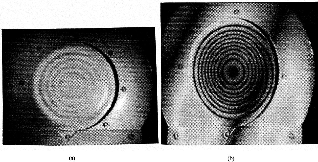
Figure 4. Image Subtraction Technique a) Original Hologram b) Enhanced Hologram
