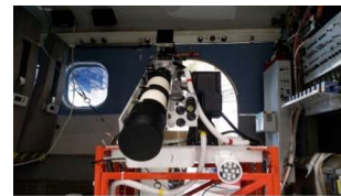
Airborne demonstration of a quantum key distribution receiver payload Christopher J. Pugh, et al, arXiv:1612.06396 [quant-ph]
