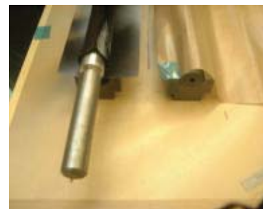
Preform in the mould before closing (With titane sheet)
