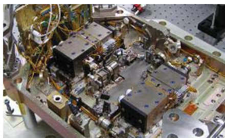
Fig. 5. Pre and Power Amplifier Subunits.
