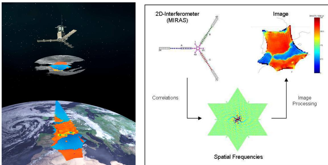
Fig. 1. Illustration of the SMOS measurement principle
