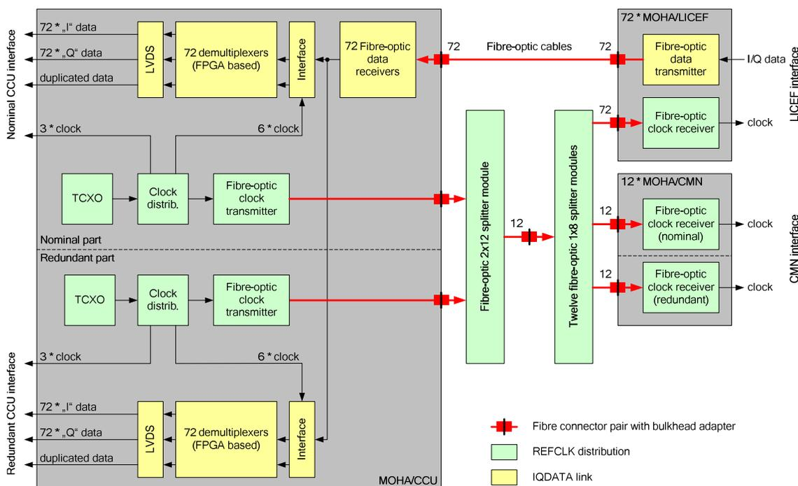
Fig. 2. Block diagram of the MIRAS Optical Harness
