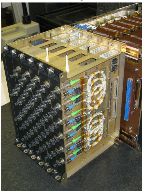
Fig. 3. MOHA module in CCU, flight model, during integration with CCU
