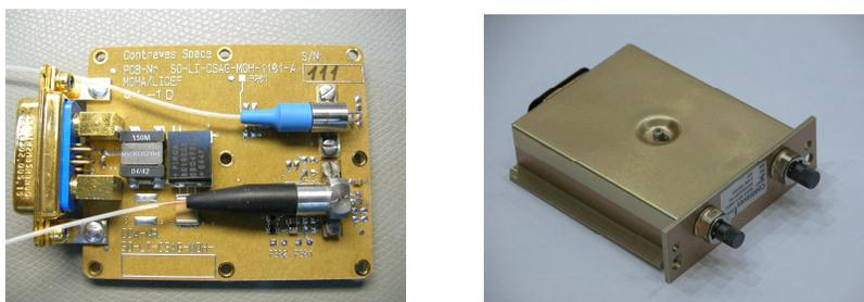
Fig. 5. MOHA module in LICEF, flight model
