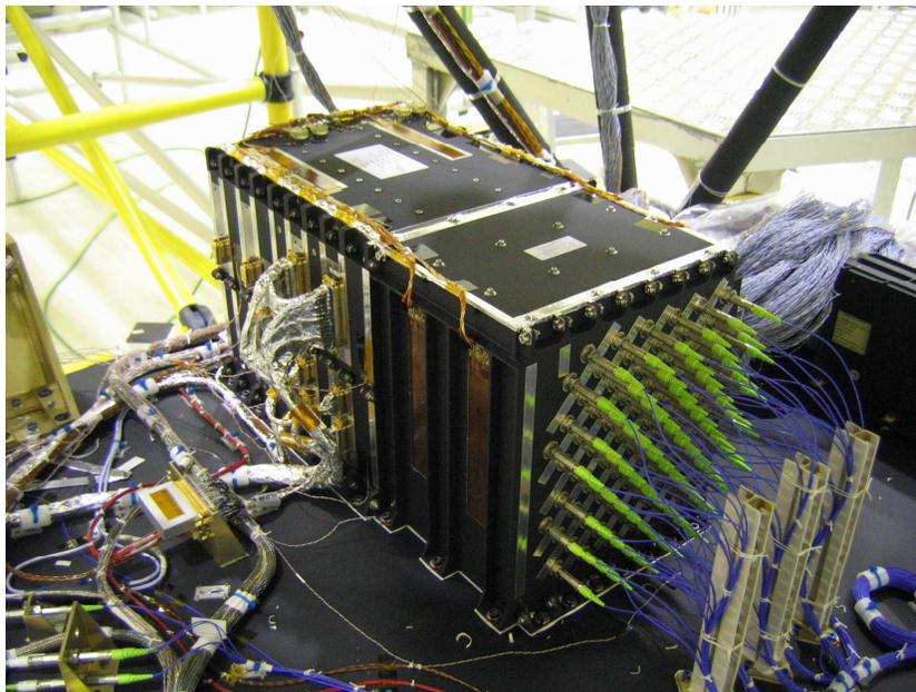
**Fig. 6.** The CCU and its MOHA part mounted on the MIRAS hub
