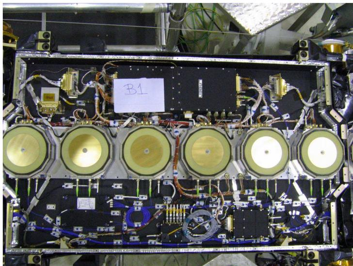
**Fig. 7.** A MIRAS arm segment with 6 LICEF, 1 CMN, and a fibre-optic 1x8 splitter
