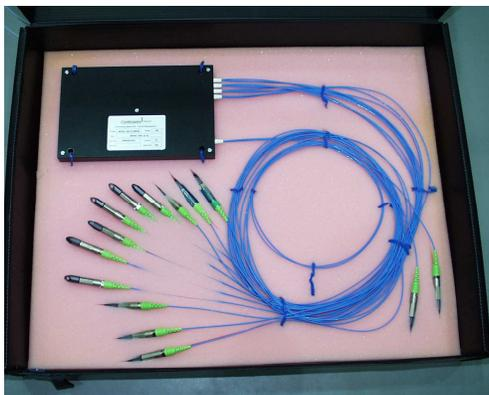
Fig. 4. MOHA fibre-optic 2x12 splitter, flight model
