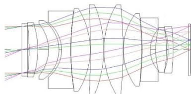
Fig.6. The layout of the co-imaging lens
