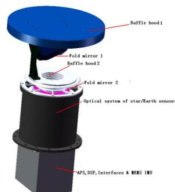
Fig.4. CANS prototype example in whole.
