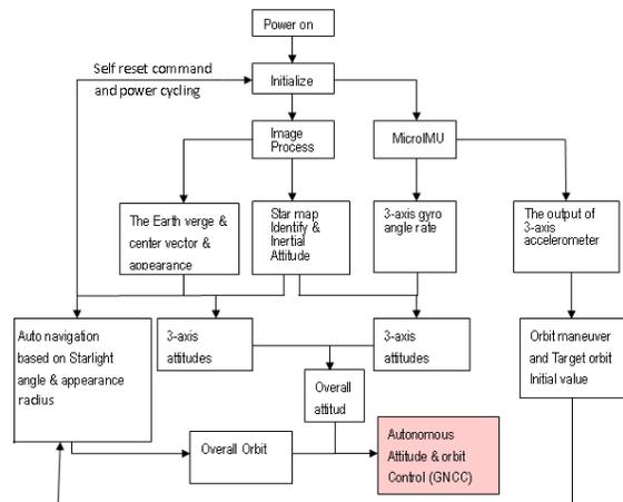
Fig.10. The CANS mode diagram
