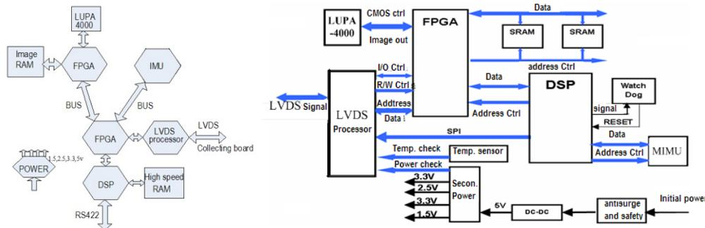
Fig.8. CANS electronical system principle diagram Fig.9. The inside information flow and structure
