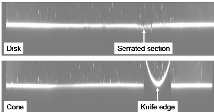
Fig. 5: Images of the diffraction fringes after the polar transformation
