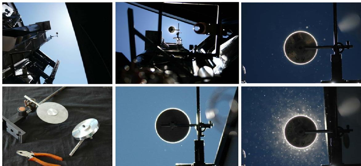
Fig. 2: Top panels: two views of the setup at Pic-du-Midi observatory and an image of the diffraction by the barrel occulter. Bottom panels: the serrated disk and the polished cone (left), an image of the diffraction by the serrated disk (center) and an image of the diffraction by the simple disk with a flurry of flying snow (right).
