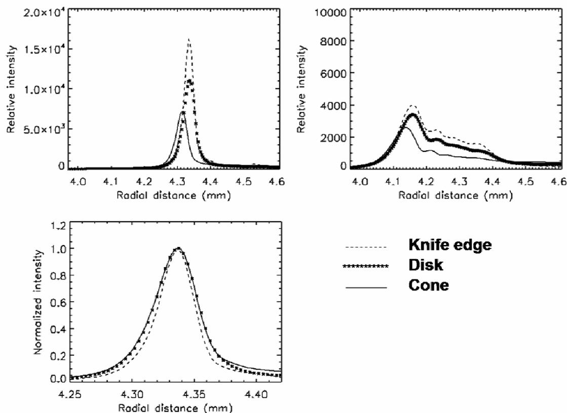
Fig. 6: Averaged radial profiles of the fringe corresponding to the knife-edge, the simple disk and the cone. The top panels correspond to focused (left) and defocused (right) cases. The bottom panel display the (focused) profiles after normalization and centring.
