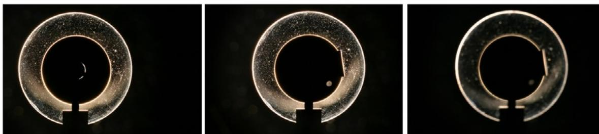
Fig. 4: Images of the diffraction fringe of the simple disk (left panel) and of the cone, both focused (middle panel) and focused at infinity (right panel).
