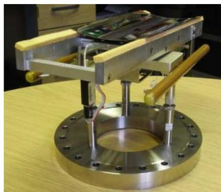
Fig. 2. Optic support structure
