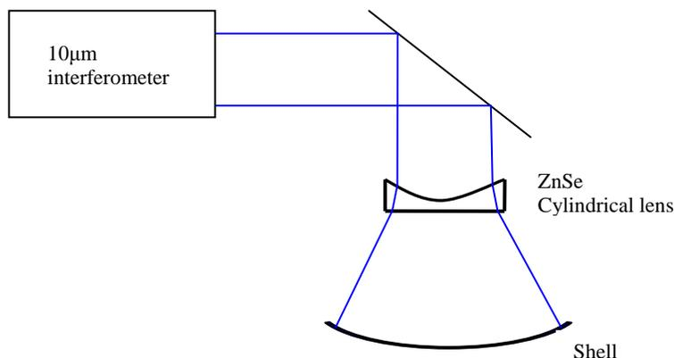
Fig. 12. Interferometric test setup
