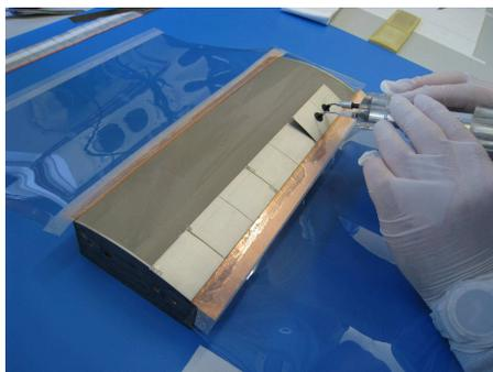
**Fig. 9.** Placement of actuators on optic
