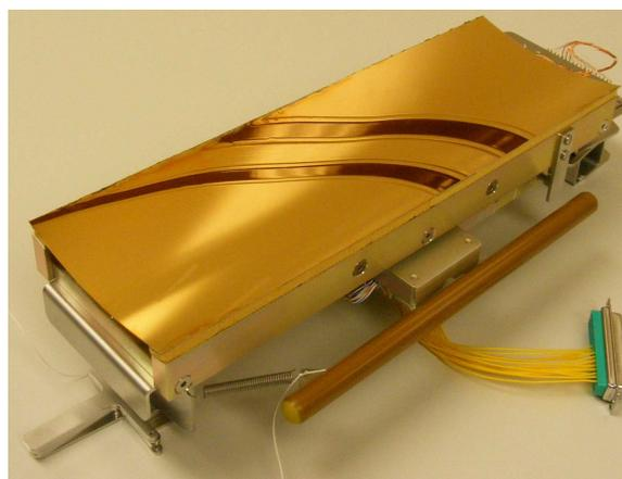
**Fig 11.** Prototype optics on its alignment mount.
