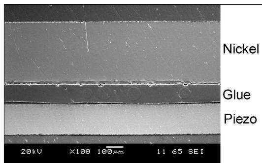
**Fig. 8.** Cross section of test piece showing glue layer
