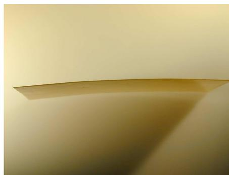
**Fig. 6.** Side view of single PZT actuator
