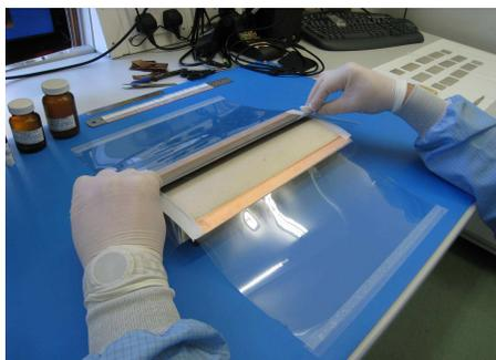
**Fig. 7.** Glue layer being applied to back of optic
