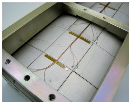
**Fig. 10.** Close up of back of optic showing wiring
