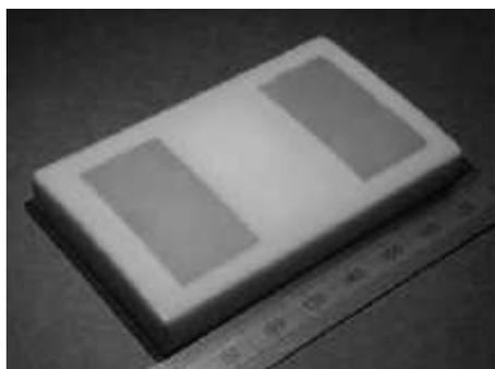
**Fig. 5.** PZT actuators on former
