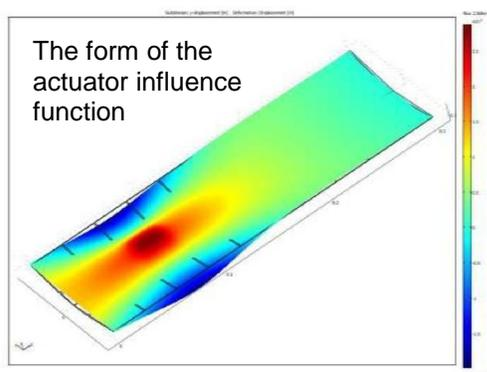
Fig. 1. FEA model of actuator influence function
