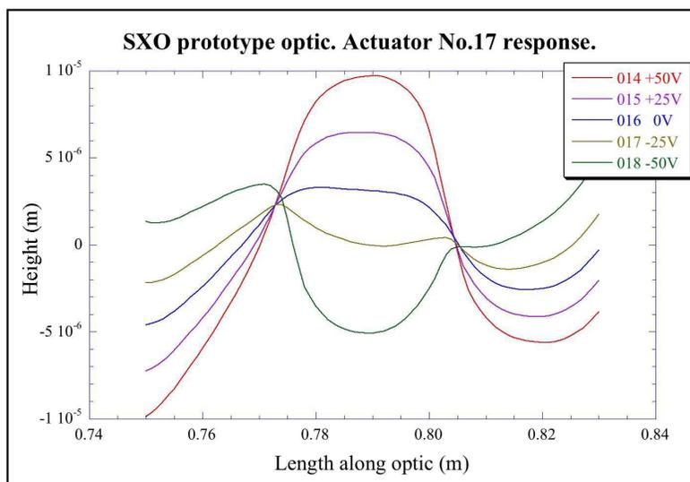
Fig. 11. Long trace profiler measurement of a single actuator at various voltages
