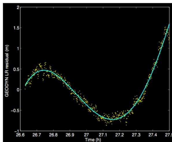
Fig. 4. Sample one-way laser ranging data from GGAO to LRO
