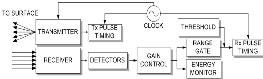
Fig. 2 LOLA Instrument functional block diagram
