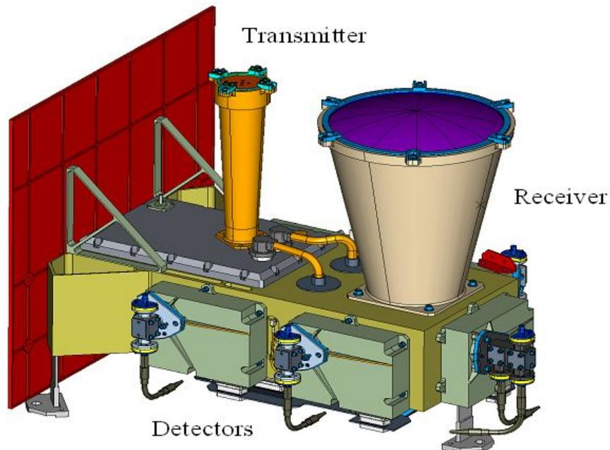
Fig. 1 LOLA Instrument Diagram
