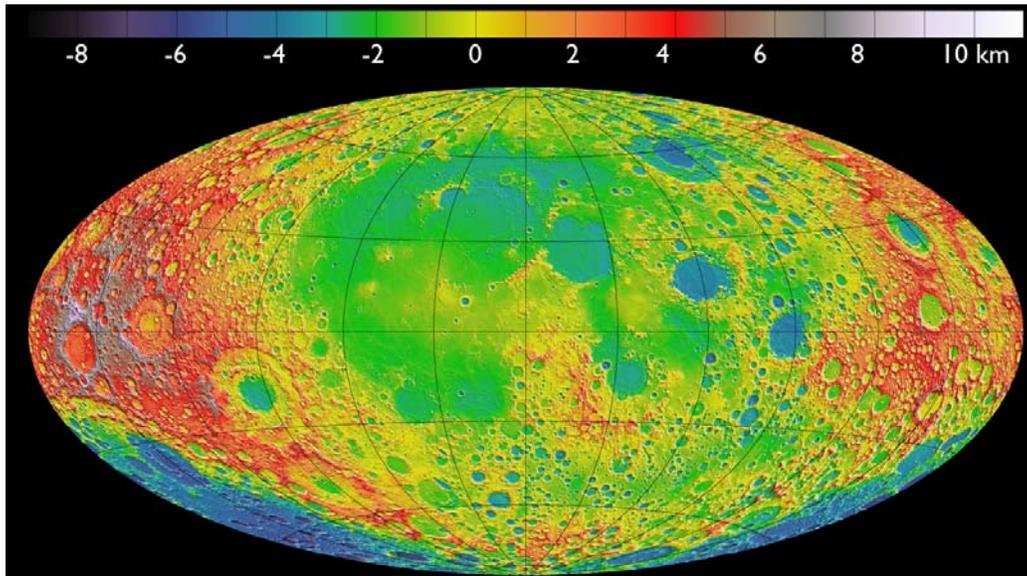
Fig. 5. Lunar topographic map with the first 1 billion LOLA measurements,
