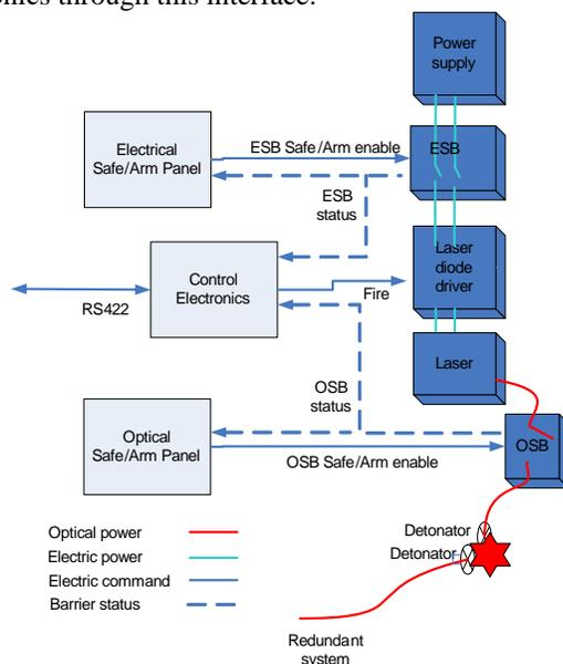
Fig.2. Opto-Pyrotechnics safety architecture
