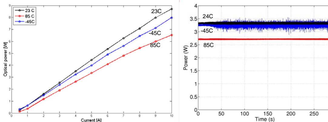
Fig. 5. Emitted laser power (power vs. current on the left; at 4A drive current and vibration on the right)
