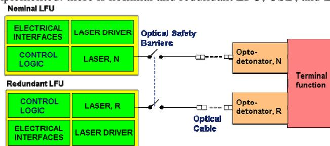
Fig. 1. Opto-Pyrotechnics system architecture
