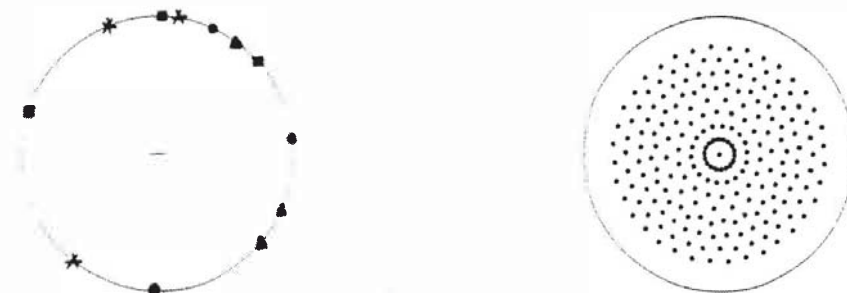
Fig. 3 : Configuration with four triplets and 9 rotations and the corresponding frequency coverage.
