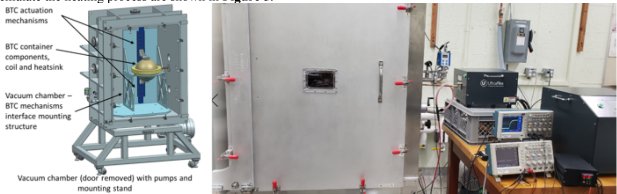
Figure 4: The brazing chamber prototype and its control hardware. Left: Design rendering, and Right: Photo of the hardware.
